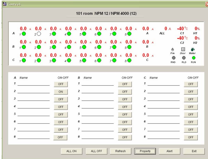
Picture 4.2.4-3. NPM 4000/5000 control managing window
