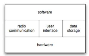
The design of the CNS is based on three main layers: the hardware layer, which consists of all different hardware parts and the interconnection from these parts to the main processor. The second layer is the interface layer, which implements all the hardware-specific software parts. This layer also gives room to the map and address databases. The final layer is the main software loop.
